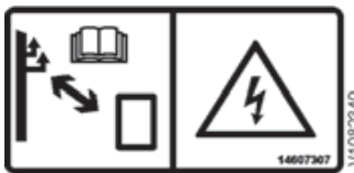
32 Electric power lines, minimal clearance
