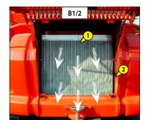
Check to see if the fins are damaged. Bent fins can be straightened using a "comb".
