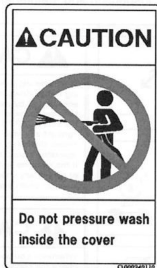
(50) High-Pressure Washing Within Cover Prohibited (CL000240110)
